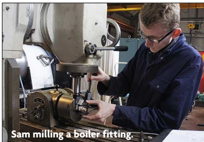
Sam milling a boiler fitting.
