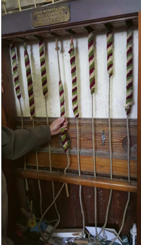
The hand pull ropes called The Ellacombe apparatus allows one person to chime all the bells.
